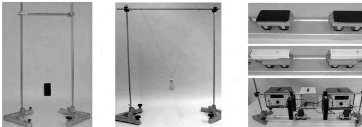
Fig 2.1: Examples of the use of MDETs replacing the traditional setup in mechanics courses: a simple pendulum with a Smartphone measuring the amplitude of oscillations (left) versus a conventional version (centre). On the right: one-dimensional collision testing the momentum conservation: with a couple of Smartphones (right-top), of WiiMote (right-centre) and conventional (right-bottom) [Hochberg, 2016].
